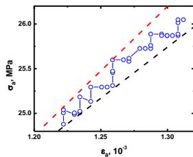
Figure 7: Detailed information within 1 MPa axial stress ( $\sigma_a$ ) for Idaho Gray sandstone. Open circles with solid lines show step-like stress-strain relation; dashed lines display the bounds for the points at the initial dynamic frictions and after dynamic frictions.
