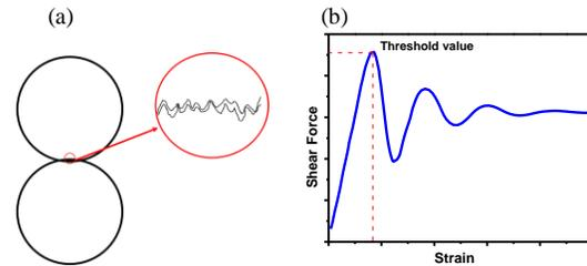
Figure 6: (a) grain contact model with randomly distributed asperities on the surface (modified after Brilliantov et al., 1996), (b) a model for converting from static to dynamic frictions (modified after Farkas et al., 2005).
