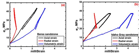
Figure 3: Stress-strain relations in the whole process for (a) Berea sandstone and (b) Idaho Gray sandstone.
