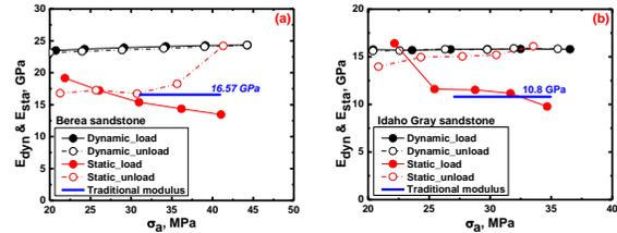
Figure 5: Static ( $E_{sta}$ ) and dynamic ( $E_{dyn}$ ) Young's moduli vs. axial stress ( $\sigma_a$ ) during triaxial load and unload for (a) Berea sandstone and (b) Idaho Gray sandstone.
