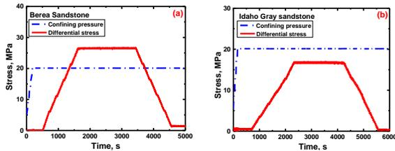
Figure 2: Experimental procedures for (a) Berea sandstone and (b) Idaho Gray sandstone.
