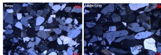
Figure 1: Thin section images for two samples, (a) Berea sandstone is composed of angular quartz mainly with point contacts, (b) Idaho Gray sandstone is composed of angular quartz and feldspar with surface contacts.
