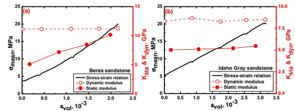
Figure 4: The mean stress ( $\sigma_{mean}$ )-volumetric strain ( $\varepsilon_{vol}$ ) curves under hydrostatic load, and static ( $K_{sta}$ ) and dynamic ( $K_{dyn}$ ) modulus vs. volumetric strain for (a) Berea sandstone and (b) Idaho Gray sandstone.
