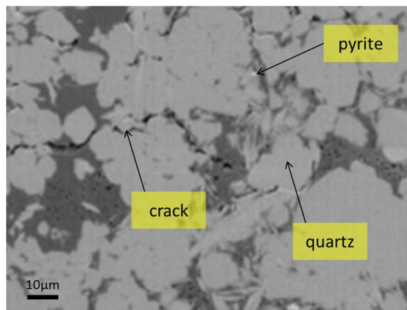
Figure 1: SEM image of a shale microstructure
