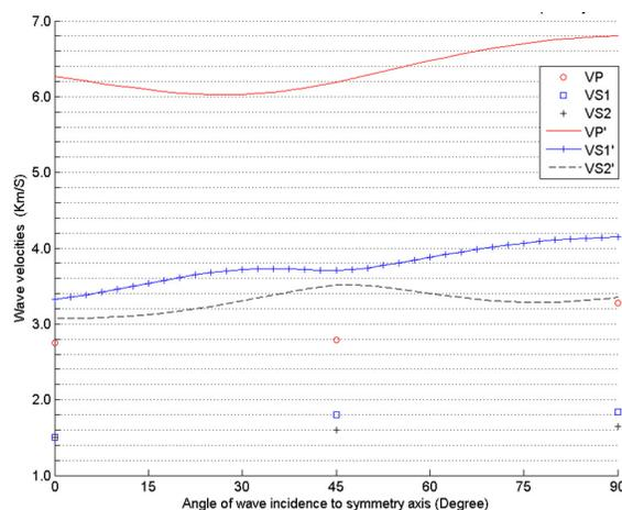
Figure 5: P, S1 and S2 velocities with different incident angles calculated from GSA modeling of pure mineral composite.
