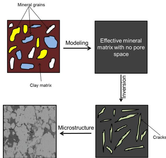
Figure 4: Schematic of the GSA method for microstructure characterization
