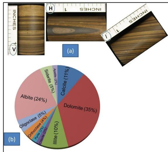
Figure 3: (a) images of the three Green River shale plugs (b) average mineralogical composition
