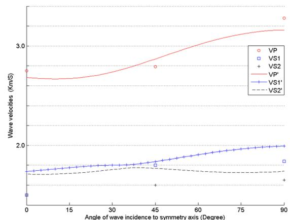
Figure 6: Comparison of calculated and experimental velocities after inversion.
