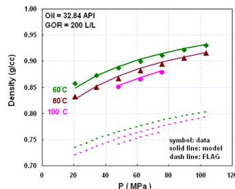
Figure 5: Density comparison of data with the models for CO<sub>2</sub>-oil mixtures with GOR 200L/L.
