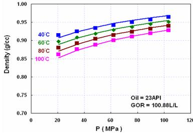
Figure 3: The density of the sample (symbol: measured data; line: calculated values by the model).
