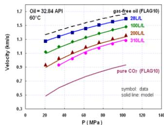
Figure 4: The measured velocity (symbols) and the prediction by the model (lines) for different GORs.
