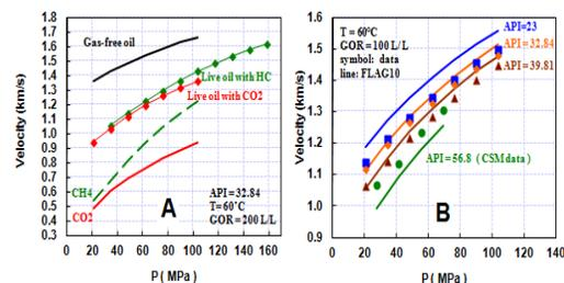
Figure 2: A. Velocities of the CO<sub>2</sub>-oil and hydrocarbon-oil; B. Velocity differences with API variation.
