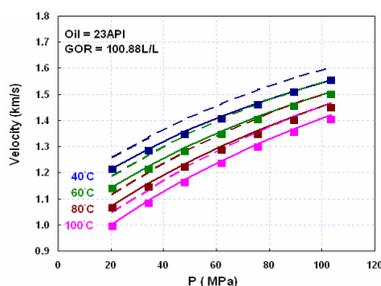
Figure 1: The measured velocity of the sample (symbol) with calculated values via FLAG (dashed line) and the model (solid line).
