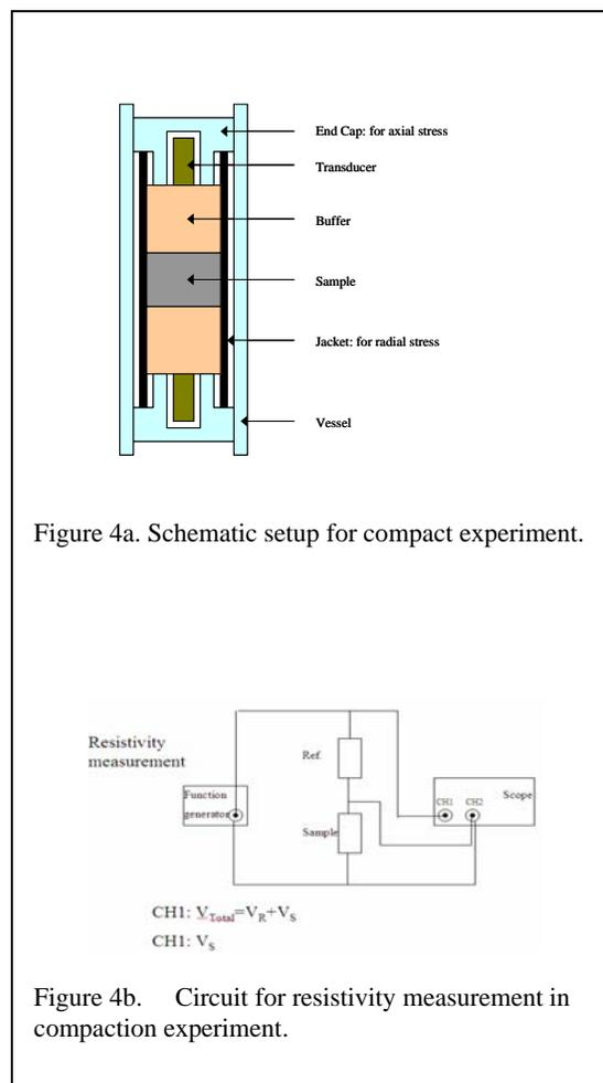
Figure 4a. Schematic setup for compact experiment.
